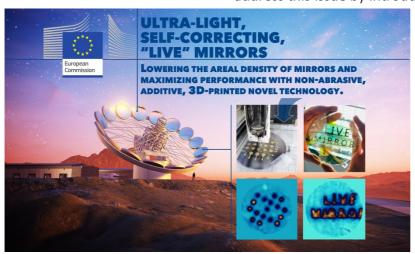
of fire-polished glass-coated sheets. These innovative mirrors will be actively supported by electro-active polymer-based actuators. By leveraging advanced manufacturing techniques and realtime control systems, the 'live mirrors' will provide superior optical quality at a fraction of the weight and cost. This disruptive solution has the potential to revolutionize
