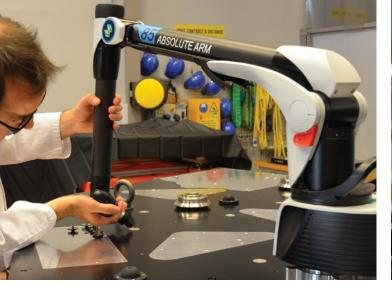
for assembly and alignment – crucial tasks such as the positioning of a mirror in relation to the interfaces. This alignment must, for some elements, be extremely precise, namely in the 10-micron range.
